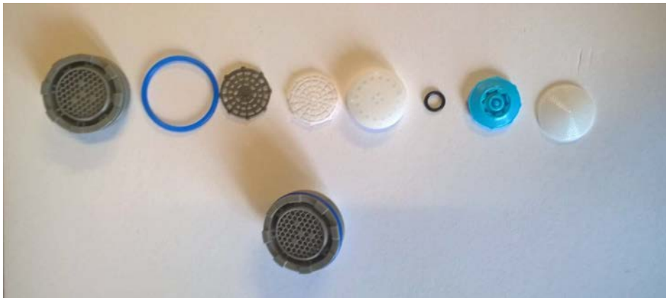
Fully dismantled flow straightener.
