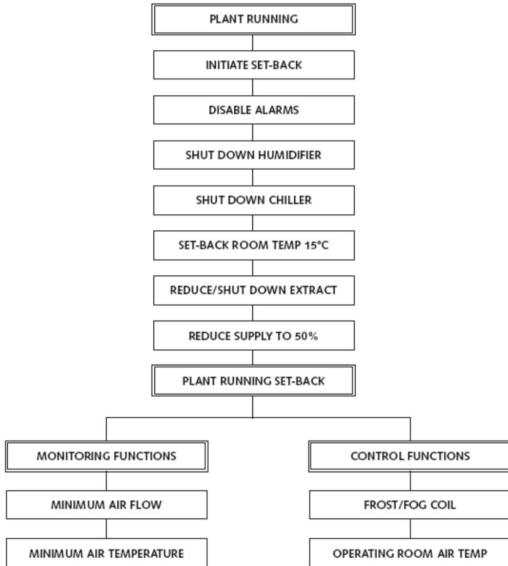
Figure 4: Plant control algorithm – set back sequence
