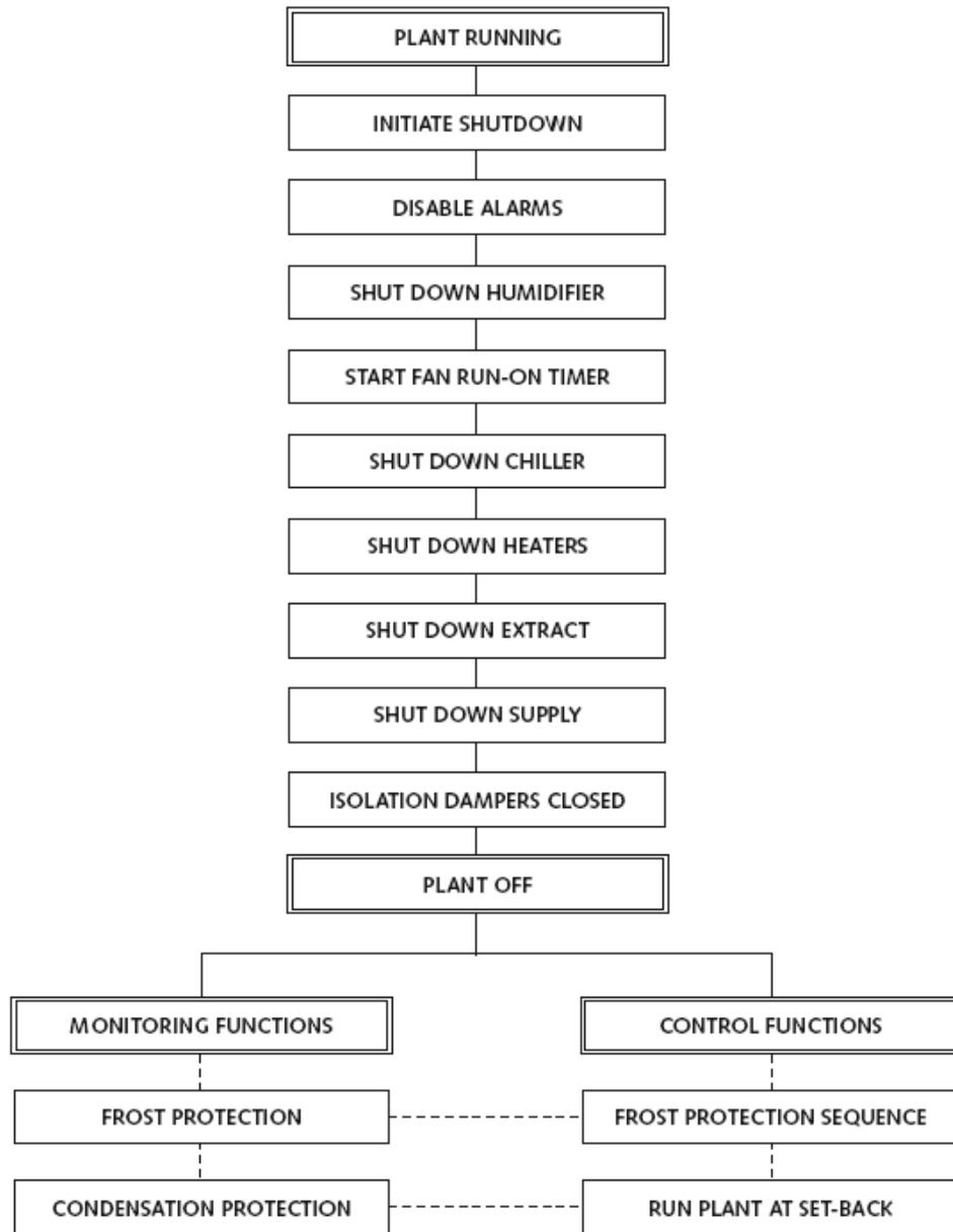
Figure 3: Plant control algorithm – normal shutdown sequence
