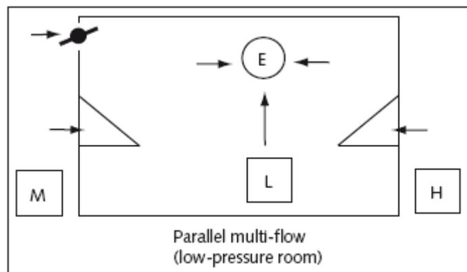
A4.15 These rooms will be either high-pressure or low-pressure with respect to the adjacent areas (see preparation lay-up room and disposal room, respectively, in [standard layout 5](#)). The pressure-relief damper is always situated between the room and area, which results in the smaller differential pressure to ensure best use of air.
