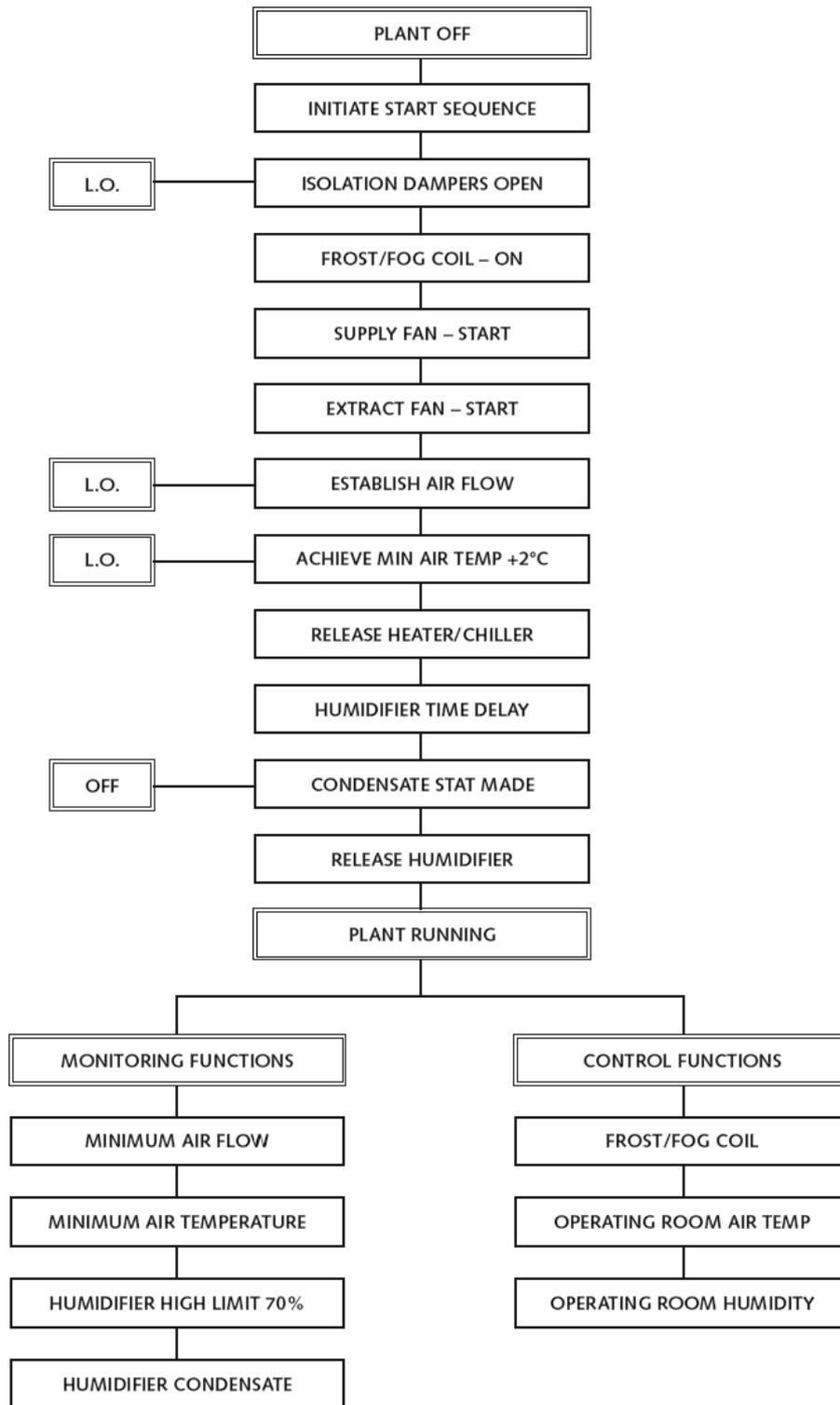
Figure 2: Typical plant control algorithm – normal start-up sequence
