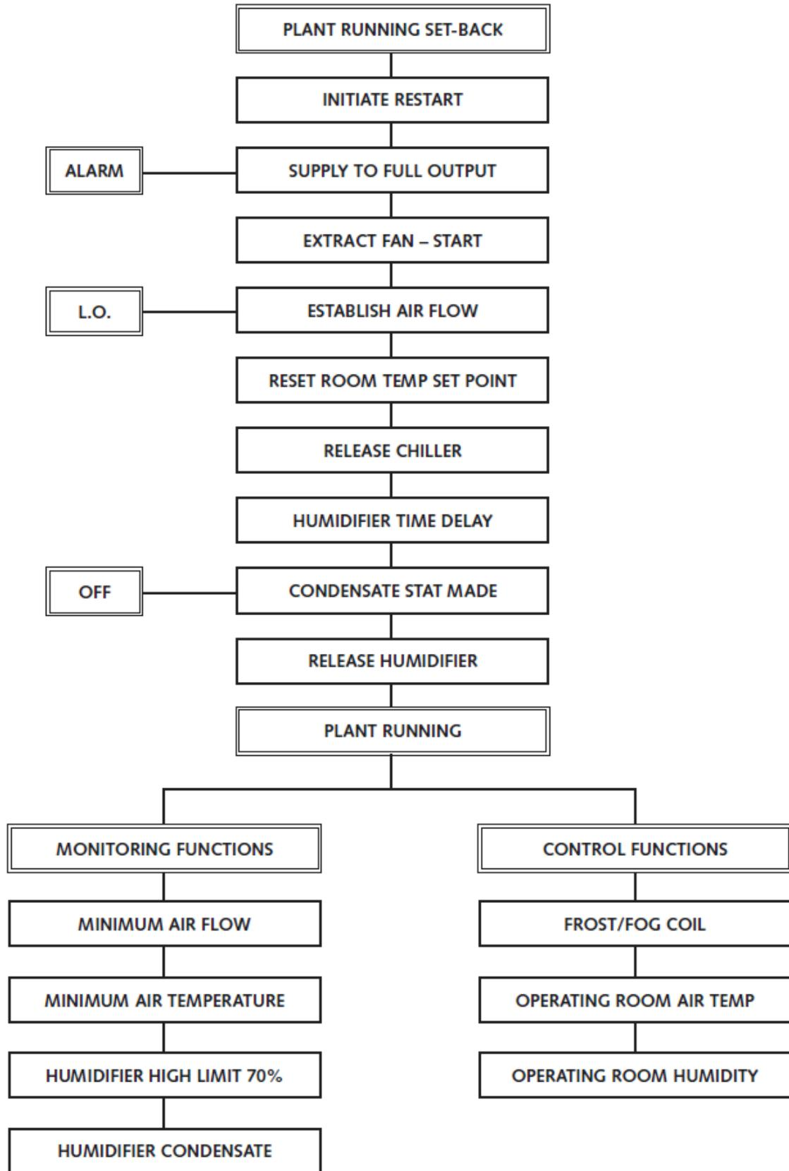
Figure 5: Plant control algorithm – restart from set-back
