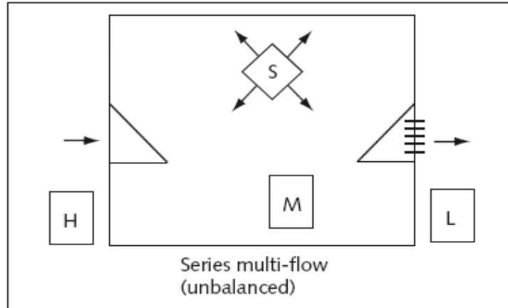
A4.21 Where the room has a net surplus of mechanical supply air, a transfer grille should be located in or adjacent to the door through which air flows outwards, and the mechanical supply flow rate to the room should be chosen to give protection when this door is open.
